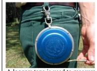
A loggers tape is used to measure distance and Tree Diameter.
