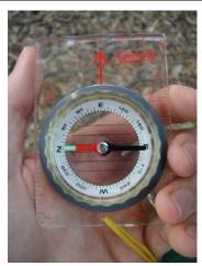
An azimuth compass showing "Red Fred in the Shed."
