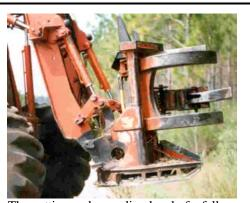
The cutting and grappling head of a feller-buncher.
